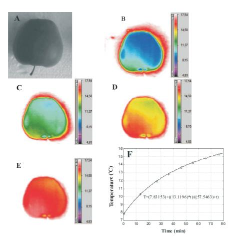
**Fig. 4.** Visible light image of a studied 'Gloster' apple (A), a sequence of thermograms during heating process (B-E), measured temperature increase and fitted curve (F).
