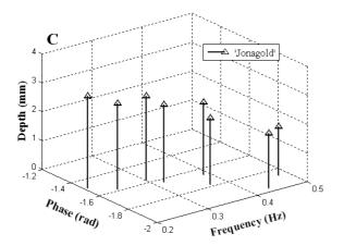
Fig. 8. Relation between bruise depth, minimum peak phase and frequency of thermal response for the studied varieties of apples.
