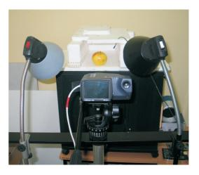
Fig. 2. Setup for early apple bruise detection study: scheme (left) and photo (right).
