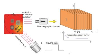
Fig. 3. Principle of pulsed-phase thermography (PPT).
